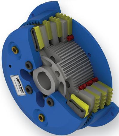
The Power Grip high speed clutch is designed to withstand the most severe applications imaginable. The heavy-duty, laminated gear tooth friction discs withstand heavy shock loads and the torsional vibrations of internal combustion engines. Drive rings are designed to fit standard SAE industrial flywheels for easy installation.
